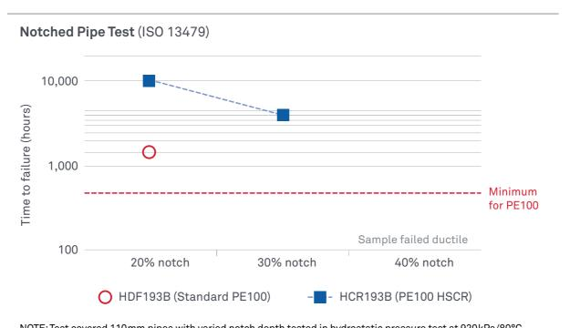
$NOTE: Test\ covered\ 110mm\ pipes\ with\ varied\ notch\ depth\ tested\ in\ hydrostatic\ pressure\ test\ at\ 920kPa/80^{\circ}C$
